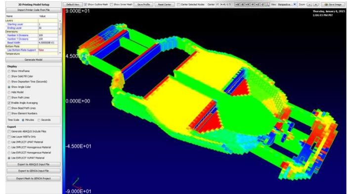
Visualize layer-by-layer the angle and time calculated in every element determined by paths printed
