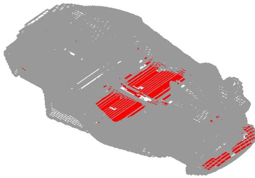
Full car model (420,000 elements, 4M dof), coupled structural/thermal/heat transfer simulated in 15 hours with 48 cpus on linux server (motherboard)
