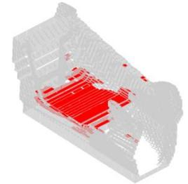
Delamination Reduced by Decreasing the Layer Deposition Time
