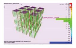
Predict macro voids distributed through the part due to errors in the printing path. These macro voids will modify the modulus, strength, and coefficient of thermal expansion of the printed part. These results are implemented into both process models and in-service loading analysis for highly accurate predictions.
