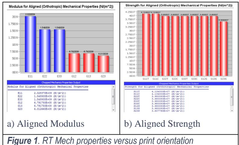
Figure 1. RT Mech properties versus print orientation
