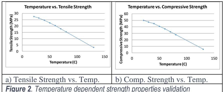
Figure 2. Temperature dependent strength properties validation
